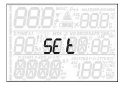
Quad Air's **SEt** menu allows you to change settings. Once inside this menu, press the **UP** or **DOWN** button to scroll between two submenus: **SEt dIVE**, where you can set parameters pertaining to the dive, and **SEt tIME**, where you can set parameters pertaining to time and date.
