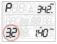
Once inside this menu, press the **UP** or **DOWN** button to change the  $0_2\%$  and observe how this affects the maximum operating depth (MOD). Then press the **ENTER** button to move on to the pp $0_2$ max and use the **UP** or **DOWN** button to change the value, again noticing how this affects the MOD. Press the **ENTER** button again to save the setting.
