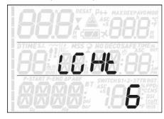
Quad Air has a backlight which can be activated in case of low ambient light. The backlight is activated by pressing and holding either of the upper buttons. During a dive, the backlight will stay on for the duration defined in this menu. You can choose between 1 and 10 seconds.
