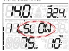
If the ascent rate exceeds 12m/min / 40ft/min at a depth below 12m / 40ft, 1 blinks as well. If a speed in excess of 12m/min / 40ft/min is maintained for two thirds or more of the depth at which the alarm was first triggered, Quad Air considers it a dive violation and the display will show the steady 1.
