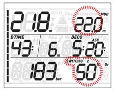
Press and hold either of the lower buttons to confirm the switch to G2: the set oxygen concentration will be displayed steadily in the lower right corner of the screen, and within 20 seconds the ascent time is updated to reflect the higher oxygen concentration in the breathing gas.
