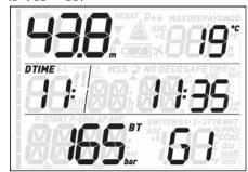
When this is displayed, press and hold either of the lower buttons to start the manual gas switching sequence. Since there is no **MOD**
