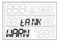
The fifth menu, **tANK RSRV**, is the value at which an alarm is triggered because you should always be at the surface before reaching this level. Furthermore, this value is used to calculate the **TTR** value (see section 3.2.5 and 3.3). This can be set individually for each tank (**G1**, **G2** or **G3**). Default values are **50bar** and **750psi**.
