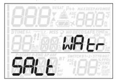
You can set the computer for **FRSH** water, **SALt** water or **EN13** calibration, depending on where you intend to dive. Setting the wrong water
