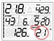
Press either of the lower buttons while this indication is blinking to initiate the gas switch: the oxygen percentage of G2 starts to blink in lieu of that of G1, and in the top right corner the MOD of G2 is displayed, also blinking.
