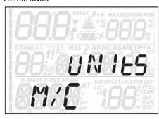
You can choose between metric (depth in meters, temperature in °C, tank pressure in bar) and imperial units. (depth in feet, temperature in °F, tank pressure in psi).
