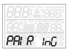
The display will show G1 in the lower right corner and the word PAIR in the middle. The top left corner shows the letters nP (Not Paired) or P (Paired) to indicate the current status of that channel. Use the UP and DOWN buttons in case you are trying to pair channel G2 or G3.
