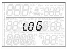
Quad Air can record the profiles of approximately 100 hours of diving, at a sampling rate of 5 seconds. The information can be transferred using the optional USB clip to PC via the Dive Organizer software or to a Mac via the Divers' Diary software. In addition, Quad Air can show most of the information directly on the display.
