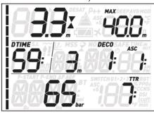
A SAFETY stop is generated as soon as the depth of the dive exceeds 10m / 33ft. It has a duration of 3 minutes and it is carried out between depths of 6m / 20ft and 3m / 10ft at the end of a dive prior to surfacing. Such stop is NOT mandatory but HIGHLY RECOMMENDED.
