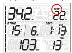
Upon reaching the optimum range for carrying out a deep stop (+/- 1m /3ft of the displayed depth), the deep stop itself will be shown in the top right corner with the label **DEEP** blinking, and a countdown timer appears to indicate the progress of the stop.
