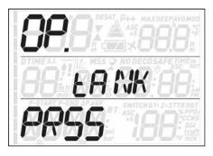
The fourth menu, **tANK WARN**, is the value at which Quad Air triggers a half tank warning. This can be set individually for each tank (**G1**, **G2** or **G3**). Default values are **100bar** and **1500** psi.
