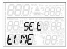
This menu allows you to set the time and date. Press the **ENTER** button and **24h** or **ampm** will start to blink. Press the **UP** or **DOWN** button to switch between the two and/or press the **ENTER** button to confirm and move on to set the hour, the minutes and the date.
