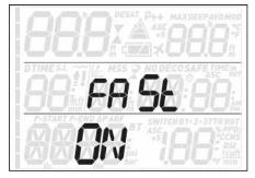
A fast (uncontrolled) ascent is defined as one in which a speed of 12 m/min / 40ft/min or higher was maintained over more than two thirds of the way up. This applies to dives deeper than 12m/40ft only. In such an event, due to the potential of harmful bubble formation, Quad Air locks the computer for 24 hours in order to discourage you from diving again. In
