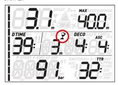
In this case, if the diver attempts a repetitive dive after surfacing, Quad Air will function only as a depth gauge and timer (bottom timer mode), and it will display  $\mathbf{x}$  on the screen.
