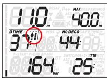
In this case, if the diver attempts a repetitive dive after surfacing, Quad Air will only function as a depth gauge and timer (bottom timer mode), and will display !! on the screen throughout the dive.
